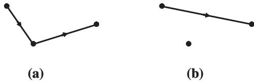
FIG. 2. (a) The two adjoining pipes of a twofold junction carry flows in opposite directions in order to satisfy flow rate conservation. (b) The two adjoining pipes can be favorably replaced with a straight one: since the total pipe length is shortened, the dissipation rate will be decreased for a fixed value of  $C_n$ .
