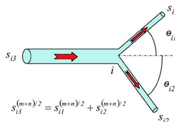
FIG. 1. (Color online) Relation between cross-sectional areas of adjoining channels in a minimal resistance network. This relation is a generalization of Murray's law.
