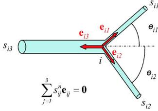
FIG. 2. (Color online) Relation between angles and cross-sectional areas of adjoining channels in a minimal resistance network. This relation is similar to a force balance equation describing the equilibrium of strings tied together and under respective tensions, or weights,  $s_{ij}^n$ .
