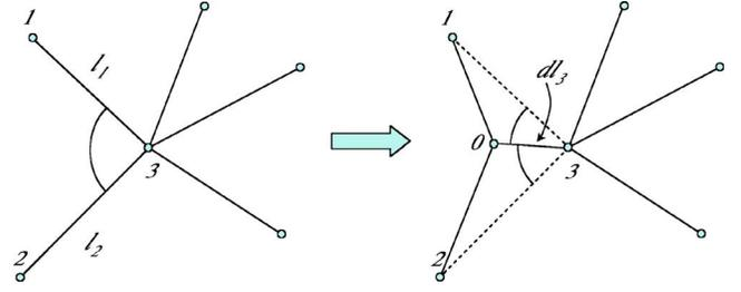
FIG. 3. (Color online) Elementary transformation of a  $N$ -fold junction to a  $(N-1)$ -fold junction plus a threefold junction. A new channel, with infinitesimal length  $dl_3$  is thus created.
