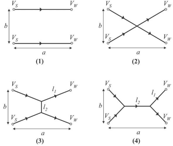
FIG. 5. Four different network configurations linking two sources to two wells, placed at the corners of a rectangle of length  $a$  and  $b$ .
